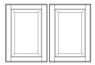
Westwind gives you the option to leave one edge of the door square while edging the other three. When ordering pair doors, the edge that is to be left square must be specified: Left (NELS) or Right (NERS). These codes should be used in the special notes column on the order form.
